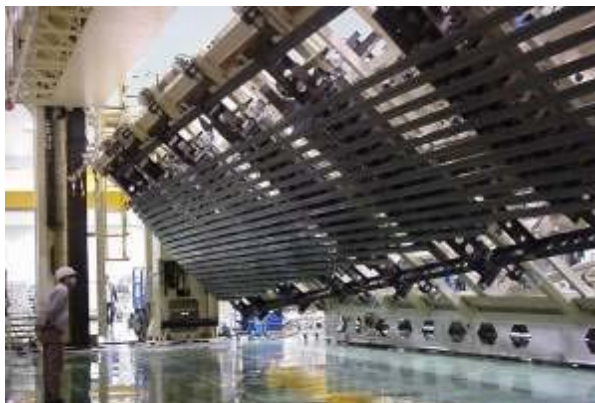
Figure 1: Placement of stringers for a stiffened CRFP skin of the A380 vertical tail plane.
